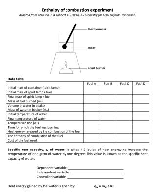
The heat gained by the water is equal to the heat released by the fuel. Therefore the heat energy released by the combustion of one mole of the fuel under investigation can be calculated using  $q_{w}$ , as long as the mass of fuel used is known.
