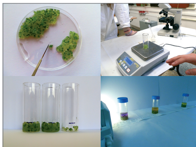
Figure 3: Working with the algal beads. Top left: Counting; top right: Weighing; bottom left: Measuring volume; bottom right: Sample layout
