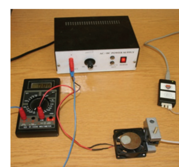
Hall-sensor for measuring rotational speed
