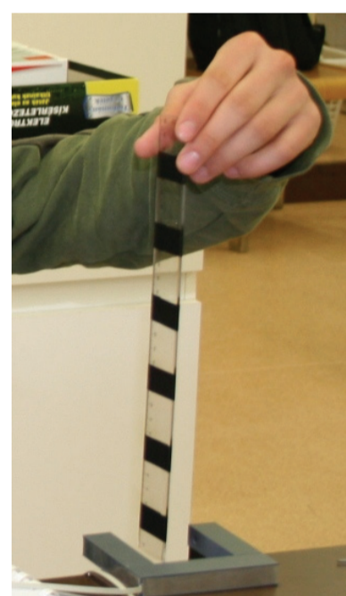
Ruler transformed into a picket fence and a photogate
